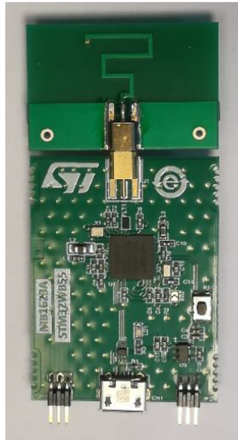
Figure 43. Monopole meandered antenna
