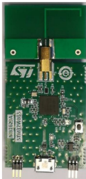
Figure 40. Monopole L-shaped antenna
